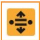
Creates a new set of corners: drags the selected roof edge out, staying parallel to the adjacent white points (see below, right)
