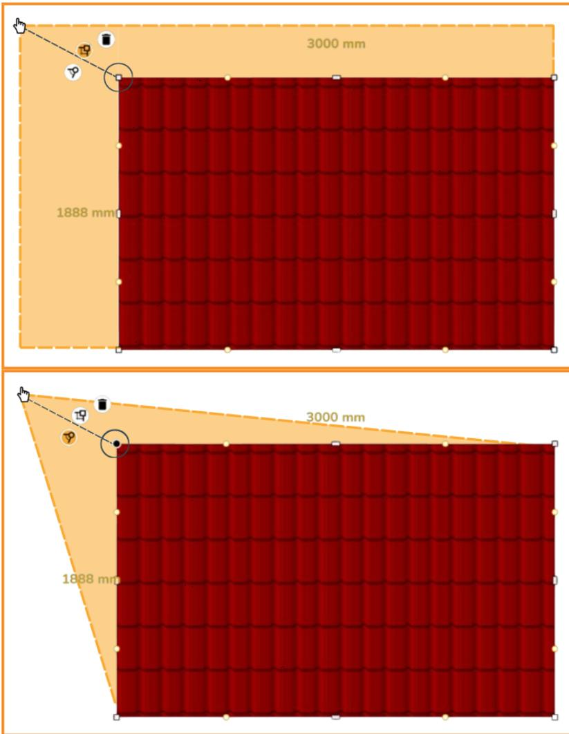
Edit roof dimensions: clicking on the white corners brings up the dimensions for the adjacent sides. If you click on this value, you will be able to input the precise dimensions for that side.
