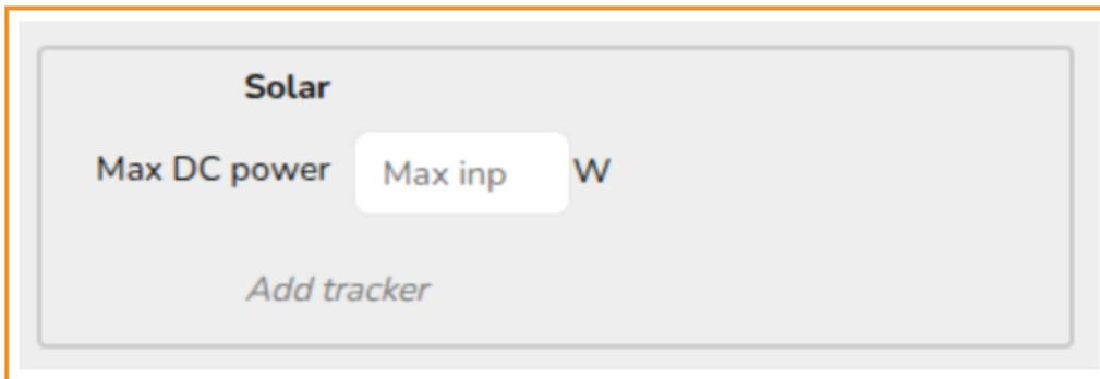
Check on the manufacturer's datasheet to see how many trackers there are for the inverter. Click the **Add tracker** option in the solar section on the right and input the relevant information. Once this is filled in you will be able to allocate the panels to the input.
