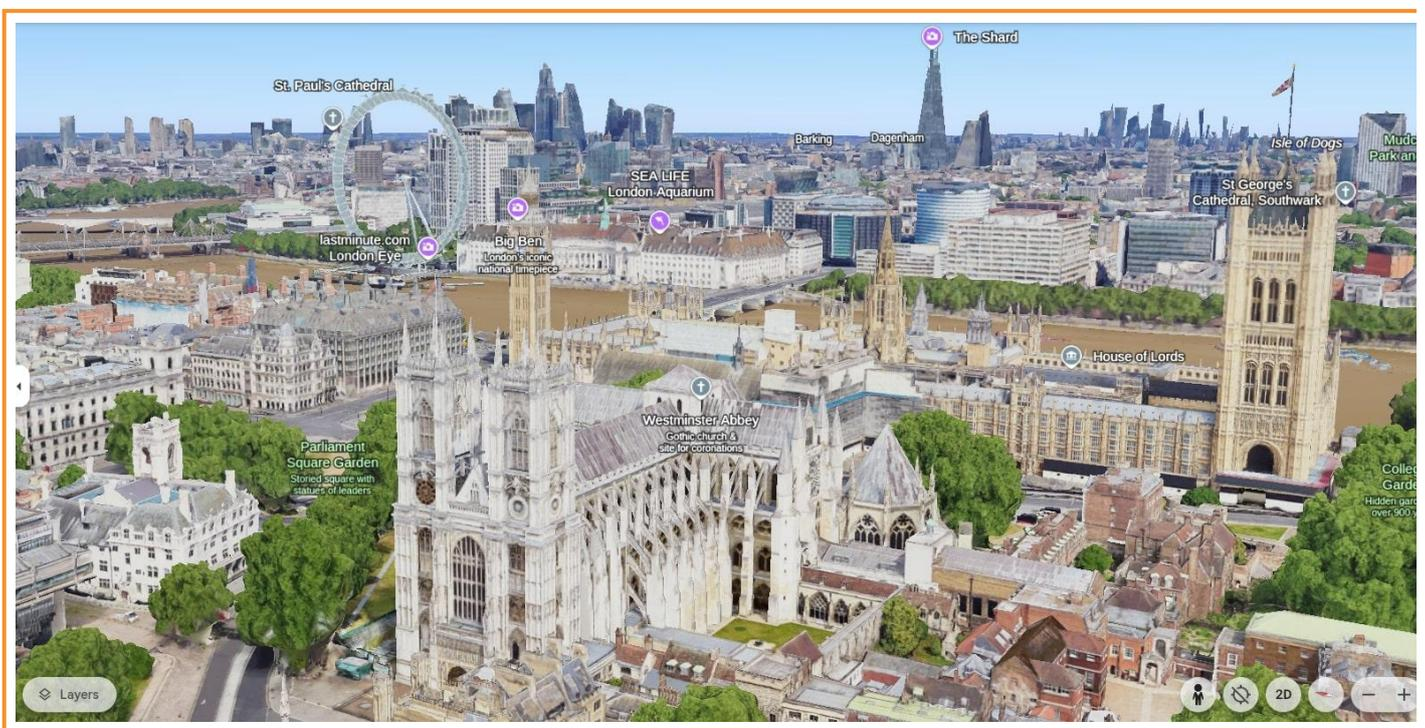
LIDAR scanning is not done by satellites, but rather by aeroplanes, and as such its coverage is much less than the coverage of normal, 2D satellite imagery. Google plans to eventually expand the areas scanned in this way, but so far they have done a pretty good job of scanning the areas where most people live, i.e. urban centres.
