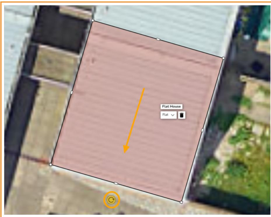
If you want to orient the panels another way on a flat roof you can use the irregular roof tool and the following steps:
